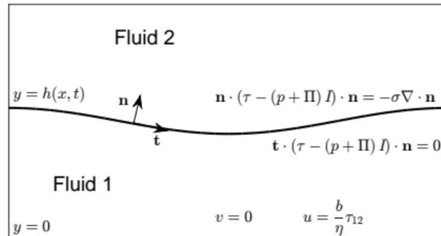
Schematic of the fluid interface and boundary conditions in the case in which  $\mathbf{F}_b = 0$ .
