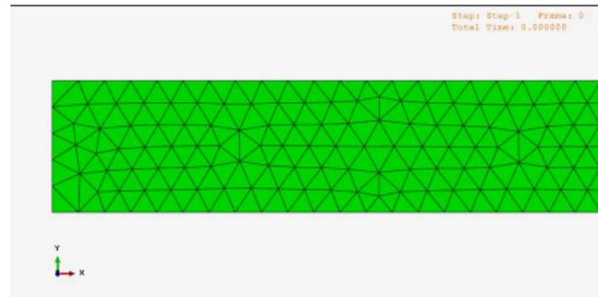
Linear finite elements with plane stress formulation. Different constitutive models considered: elastic, viscous, viscoelastic (Maxwell)
